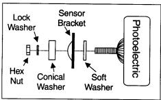
Mount the infrared safety sensors to the sensor bracket keeping the soft washer between the sensor and sensor bracket and then place the conical washer, lock washer and hex nut on the extender bolt, as illustrated.
